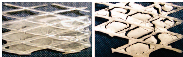
Figure 6. Picture of dried silica films synthesized with (left) CTAB:LPEI and (right) CTAB:SPEI.
